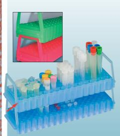
The handles of the lower rack make a perfect fit with those of the upper one, ensuring a stable unit which can easily and safely be moved around.
