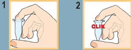
All Simport Microcentrifuge tubes offer a CLIKLOK™ seal especially designed to reduce popping where freezing, boiling, storing or shipping is required. This superior quality CLIKLOK™ system works in two stages:
