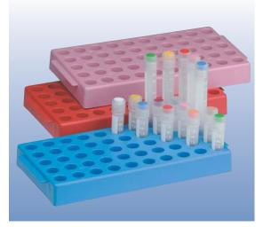
Now, with only one hand, you can easily unscrew a **Simport** Cryovial<sup>®</sup> closure. Thanks to an innovative universal locking base, the vials will securely lock in the wells of just about any rack on the market. This newly designed feature is available on all **Simport** self-standing Cryovial<sup>®</sup> tubes.
